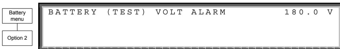
Figure 8-56: Battery test voltage alarm setup
