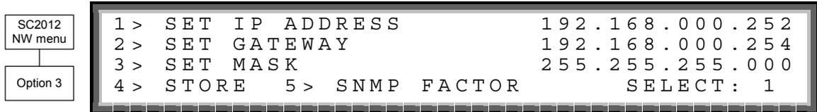
Figure 8-81: Service – SC2012 network setup menu
