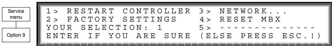
Figure 8-80: Service – SC2012 controller reset menu
