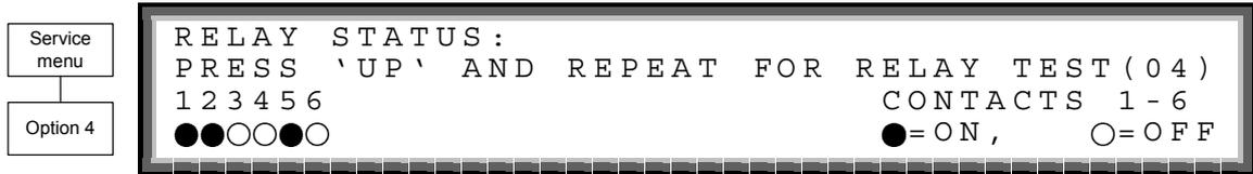
Figure 8-77: Service – setting alarm contacts
