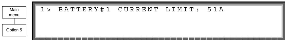
Figure 8-27: Battery current limit
