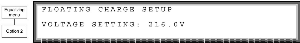
Figure 8-70: Setup – setting floating voltage
