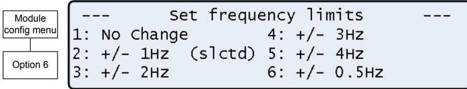
Figure 8-51: Output fine-tuning – set frequency limits
