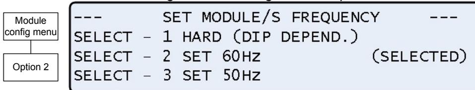
Figure 8-45: Setting the sine wave frequency
