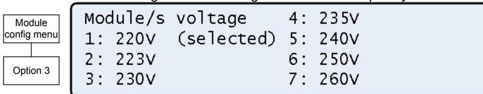
Figure 8-46: Setting the module voltage
